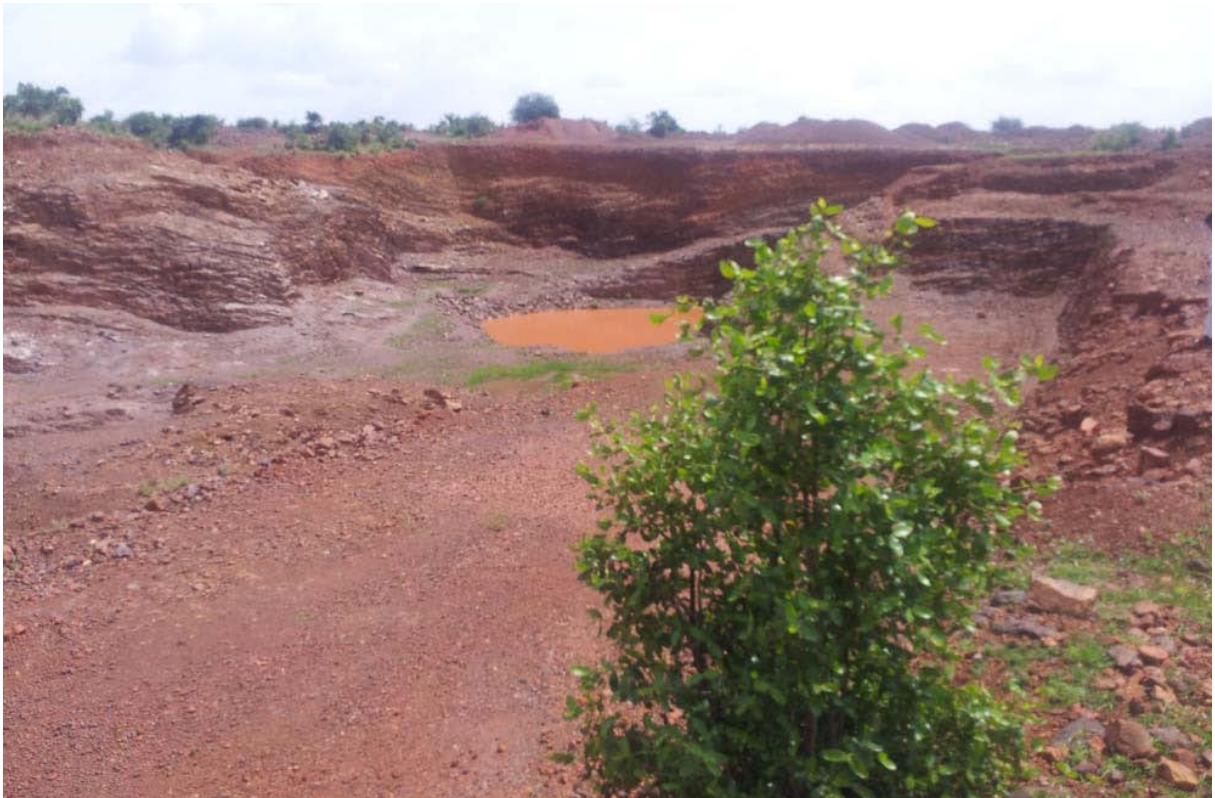
Trial Pits Showing Continuity of Bedding and Depth Persistence
